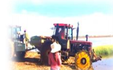
Cage wheels: sowing and spreading fertilizer on flooded land
